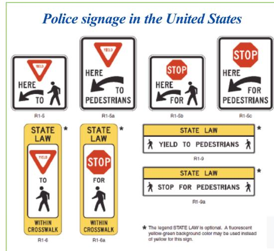
Differences exist mainly in regulatory signs for traffic in specific areas, such as pavements, cycle strips and lanes or in pedestrian areas. These signs are mainly for bicycle users and pedestrians sharing space with other users. These signs are usually made up of combinations of elements established in the Vienna Convention that are slightly modified. If a country wants to create a new regulation, the principle is that it uses the sign in the Convention, if it exists, or a variant thereof.
